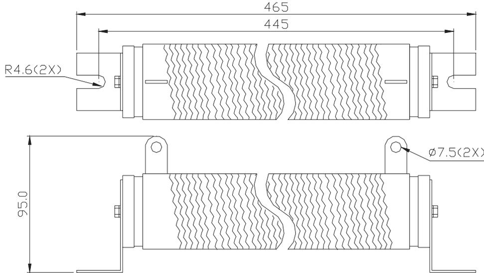
**B.1.2 Specifications for Braking Unit**
