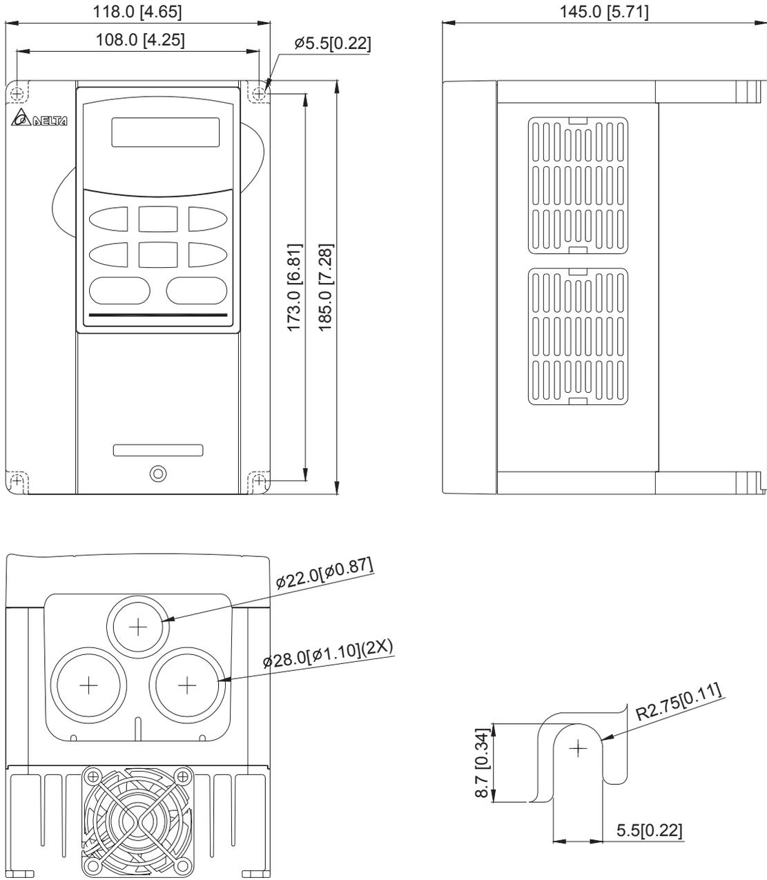
Frame B: VFD022B21A, VFD037B23A/43A/53A
