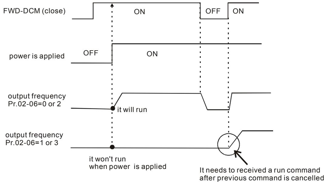
**⚠ The Line Start Lockout feature does not guarantee that the motor will never start under this condition. It is possible the motor may be set in motion by a malfunctioning switch.**
