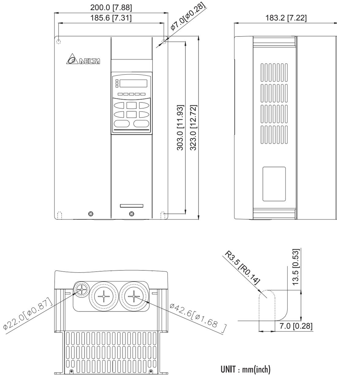
Frame D: VFD150B23A/43A/53A, VFD185B23A/43A/53A, VFD220B23A/43A/53A
