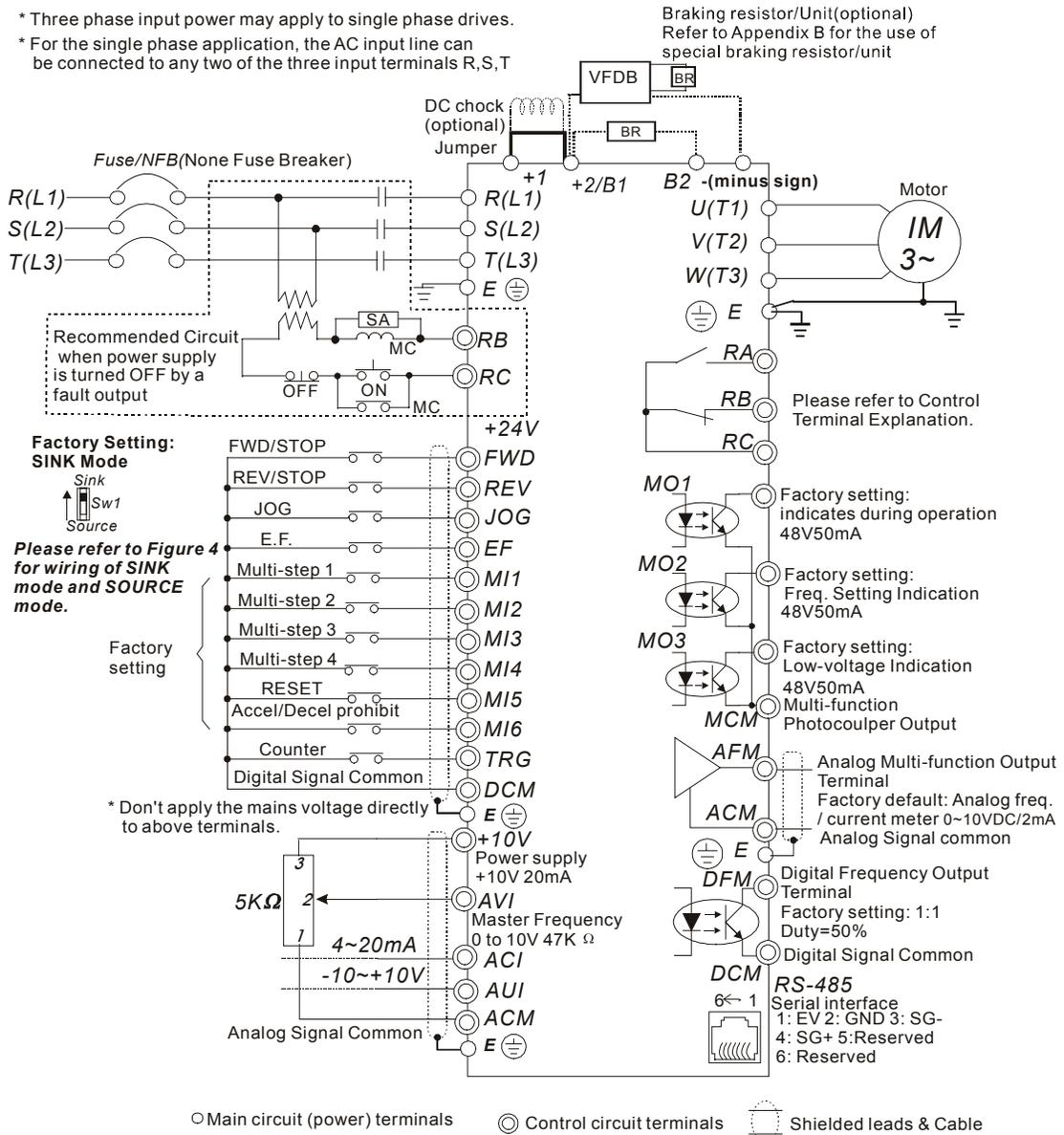
**Figure 3 for models of VFD-B Series**
