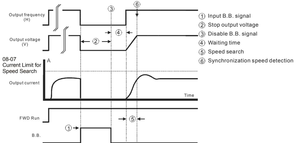
Fig 2: B.B. Speed Search with Last Output Frequency Downward Timing Chart
