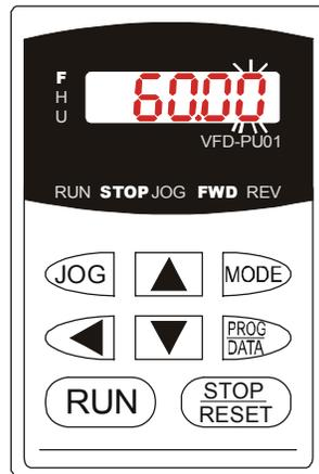
When power is ON, LEDs "F", "STOP" and "FWD" should light up. The display will show "60.00" with the least signification "0" flashing.
