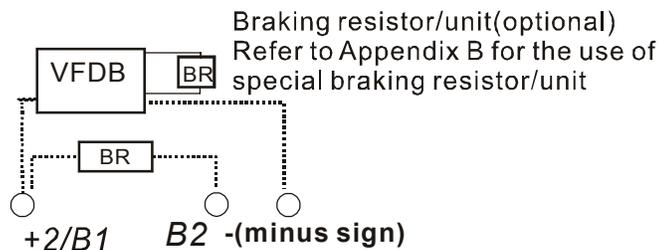
Connect a brake resistor or brake unit in applications with frequent deceleration ramps, short deceleration time, too low braking torque or requiring increased braking torque.
