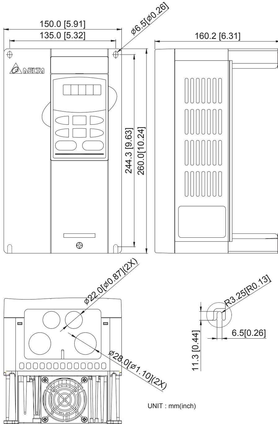
Frame C: VFD055B23A/43A/53A, VFD075B23A/43A/53A, VFD110B23A/43A/53A
