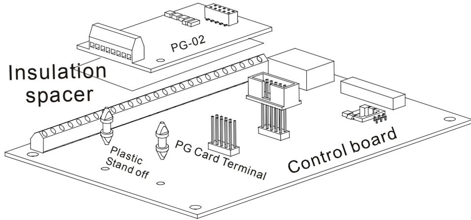
B.3.1.1 PG Card and Pulse Generator (Encoder)
