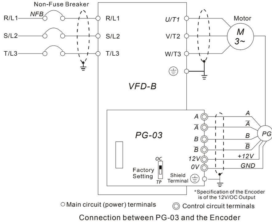
2. Connect Externally with the Encoder of 12V Power Supply and Output Signals to Additional Tachometer
