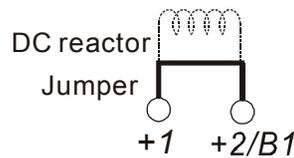
To improve power factor and reduce harmonics connect a DC reactor between terminals [+1, +2]. Please remove the jumper before connecting the DC reactor.
