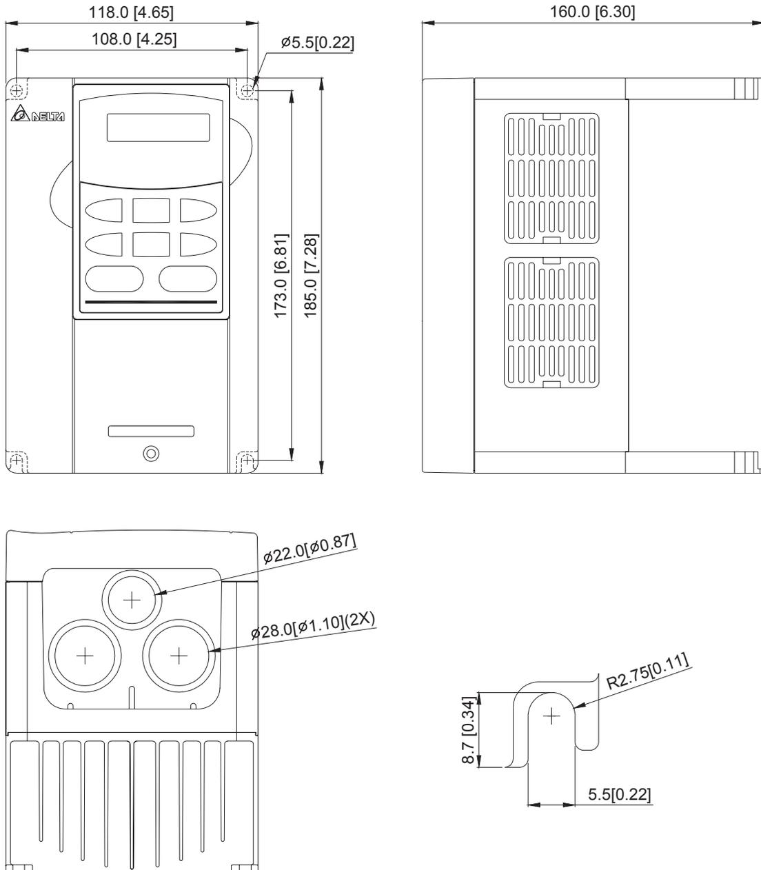
Frame A2: VFD015B21B/23B, VFD022B23B/43B/53A
