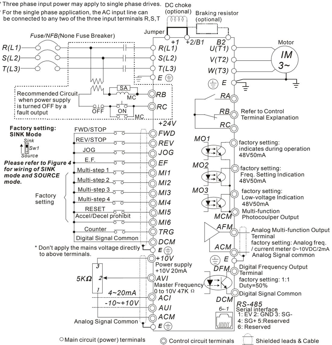
**Figure 2 for models of VFD-B Series**
