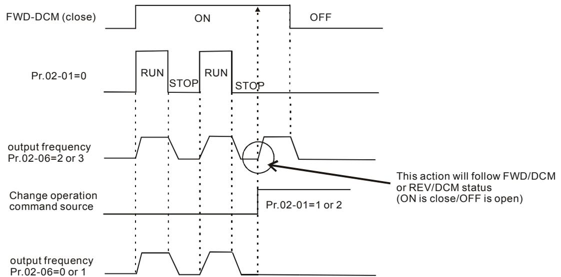
When the operation command source isn't from the external terminals, independently from whether the AC motor drive runs or stops, the AC motor drive will operate according to Pr.02-06 if the two conditions below are both met.
