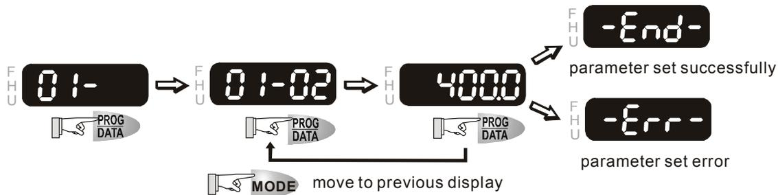
NOTE: In the parameter setting mode, you can press **MODE** to return to the selection mode.
