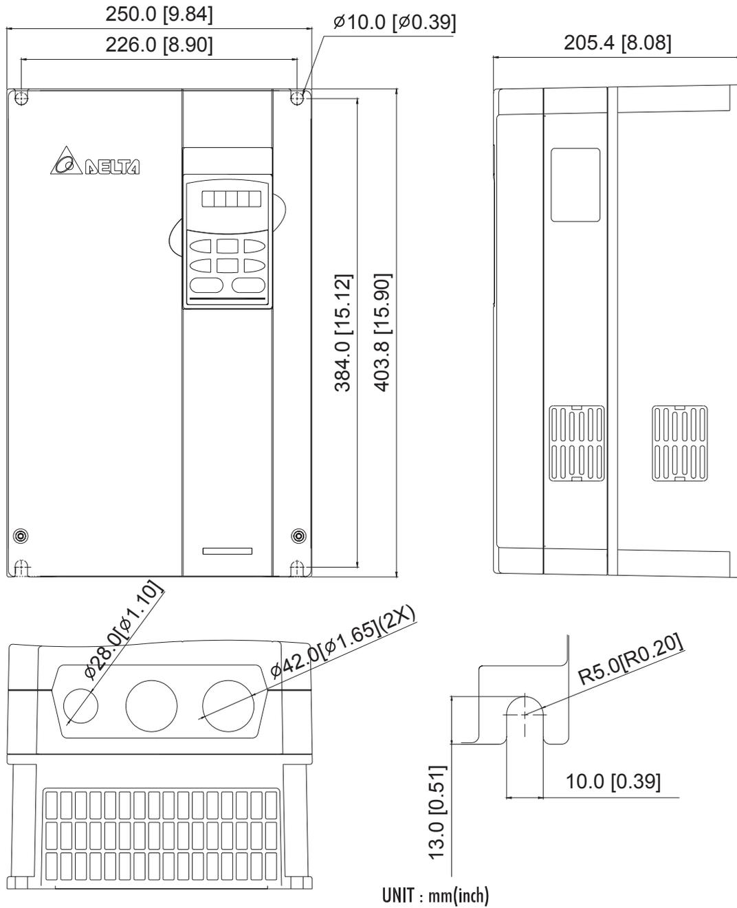
Frame E: VFD300B43A/53A, VFD370B43A/53A, VFD450B43A/53A
