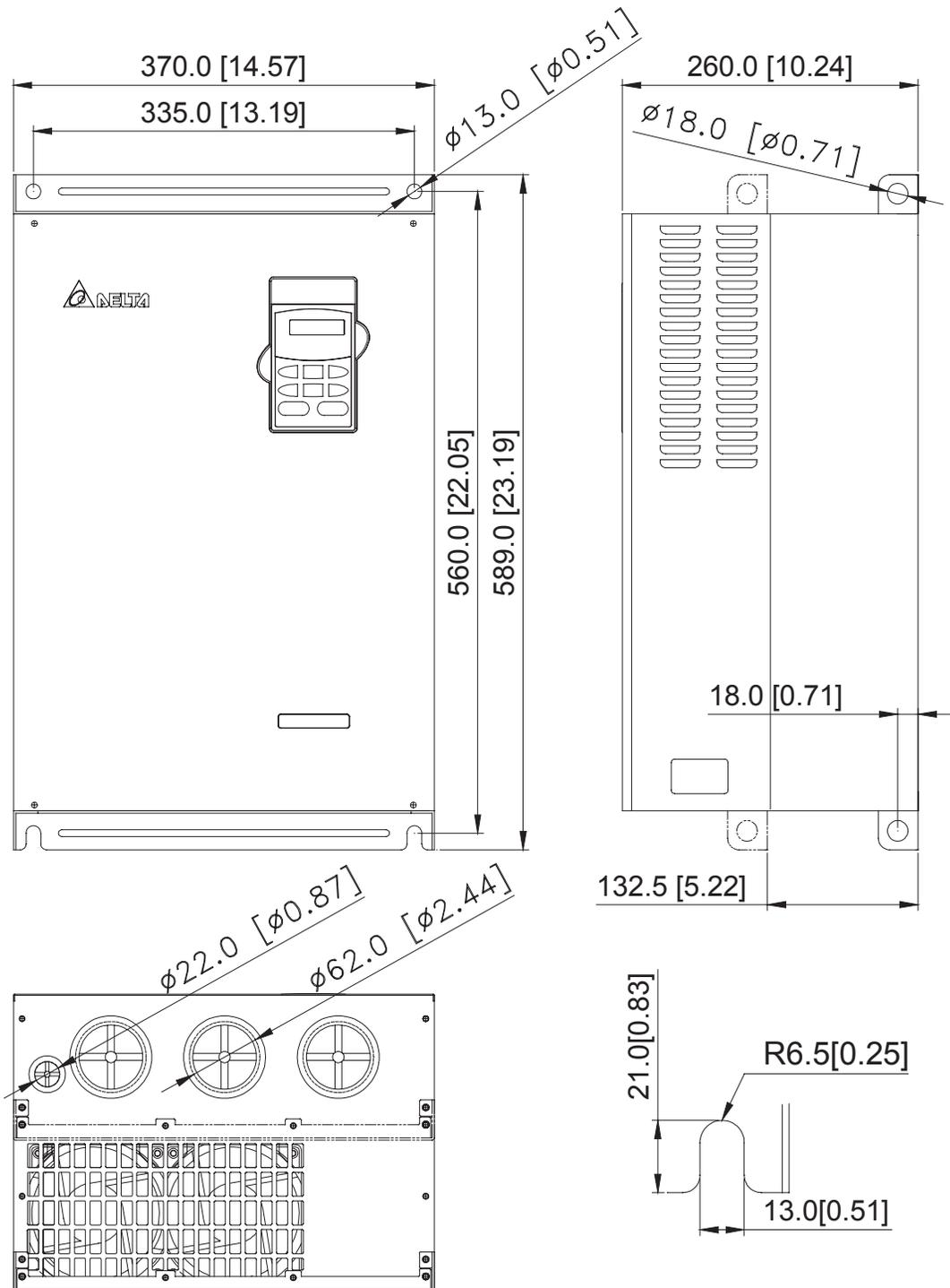
Frame E1: VFD300B23A, VFD370B23A, VFD550B43C/53A, VFD750B43C/53A
