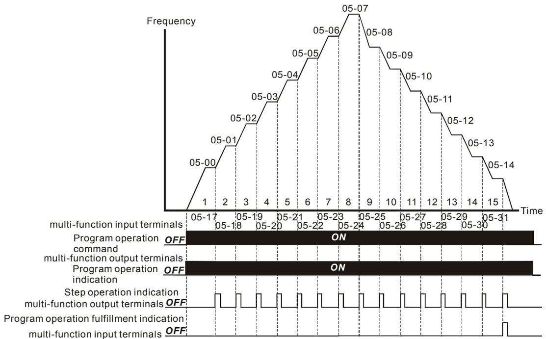
**NOTE** The above diagram shows one complete PLC cycle. To restart the cycle, turn the PLC program off and on again.
