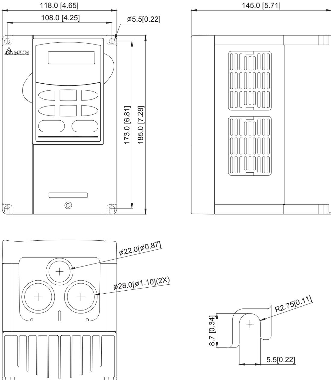
Frame A1: VFD007B21A, VFD015B21A/23A/43A/53A
