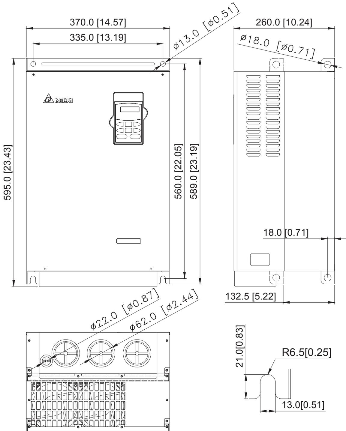
Frame F: VFD550B43A, VFD750B43A
